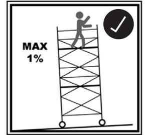
Maximum inclination for movement. Note the maximum angle allowed is defined by the manufacturer.
